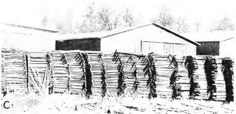
A, Oak barrel-heading stock piled for air seasoning in the form of a hollow cylinder; B, thick veneer stock end piled for air seasoning under a double roof; C, veneer stock flat piled for air seasoning
